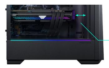
because there is enough space to install either the fans or the radiator in front of the chassis now, more clearance is available for the GPU
