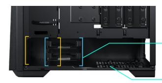
flexible HDD brackets positioning to either enable 360 radiator in the front or create more space for the PSU
