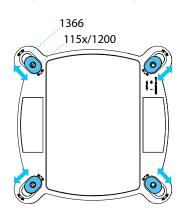
B) Secure the 4x 115x/1200/1366 Stand-offs to the motherboard and Intel Backplate
